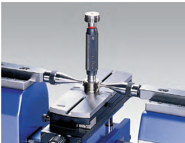
▲ Setting of threaded plug gages from diameter 1.18" to 9.84" (30 to 250mm) using table (54-196-160-0), small Ø anvils (54-190-806-0) and thread wires (54-197-007-0)
