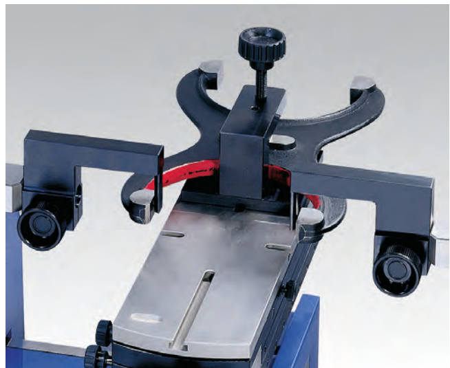
▲ Checking of snap gages from .473 to 6" (12 to 150mm) using table (54-196-160-0), snap gage holder (54-190-815-0) and L-probes (54-197-162-0)
