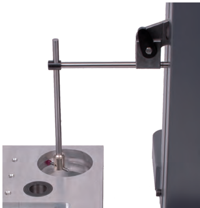
Internal groove measurements with accessories 54-199-508, 54-199-506 and 54-199-501
