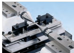
Checking of plug gages and threaded plug gages between centers up to max. dia. 1.18"/30mm, max. length 6"/150mm using table (54-197-011-0), small Ø anvils (54-197-806-0) & thread wires (54-197-007-0)
