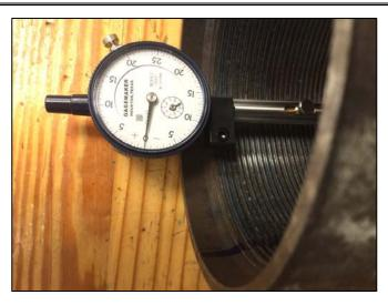
9. Roll the coupling one complete revolution and make note of the minimum and maximum indications.
