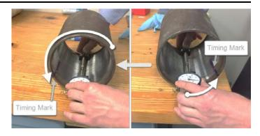
10. Determine the total sweep by subtracting the minimum indication from the maximum indication.
