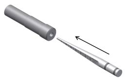
**Note:** The nozzle should be replaced when the orifice is worn more than 1/16" larger than the original orifice size, as this is the point that performance beings to dramatically decline.
