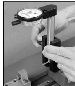
Mounting different styles of pivot arm gages
