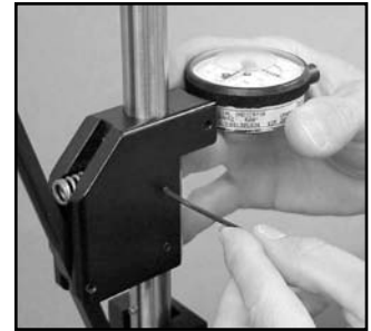
Using a 5/64" hex wrench to align the gage
