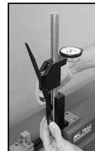
Mounting different styles of pivot arm gages
