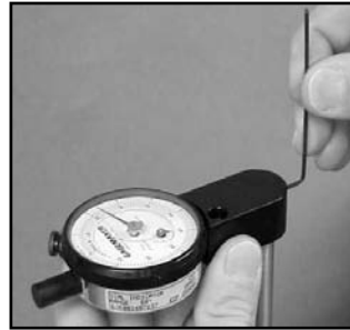
Using a 1/16" hex wrench to align the gage
