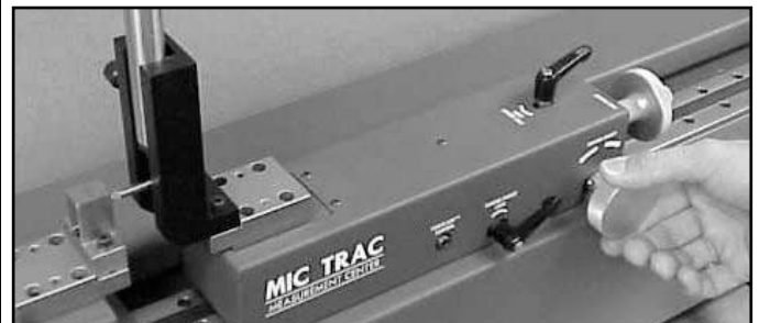
Aligning the indicator dial on different styles of pivot arm gages
