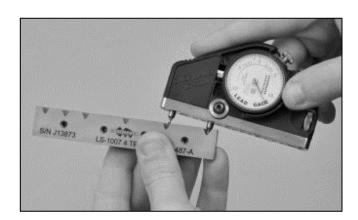
2. Place moveable contact point into the first groove of standard.
