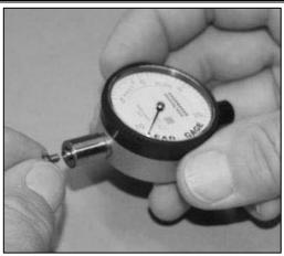
6. Place the new indicator assembly back into the body of the gage.
