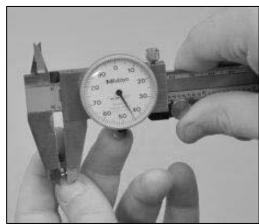
4. Install a contact point into the moveable holder at the front of the gage.
