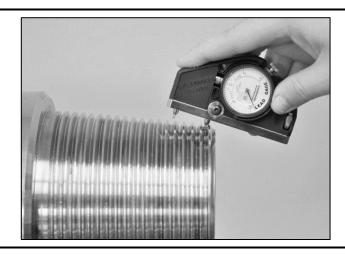
Rock the gage forward and seat the moveable contact point into the thread. Use your index finger to apply just enough pressure to maintain the gage's contact with the thread flanks.
