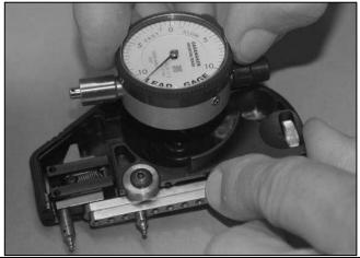
5. Replace the contact point in the new indicator with the contact point from the old indicator.
