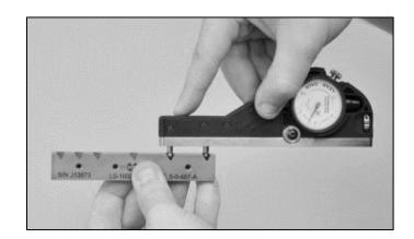
With the two contact points properly seated in the grooves of the standard, sweep the moveable contact point from side to side in order to obtain the smallest indicator reading (needle changes direction).
