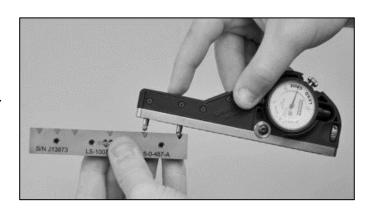
2. Place moveable contact point into the first groove of standard.
