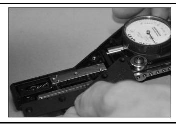
5. Lift the indicator out of the gage body.
