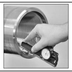
Rock the gage forward and seat the moveable contact point into the thread. Use your index finger to apply just enough pressure to maintain the gage's contact with the thread flanks.
