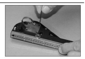
3. Remove the five screws on side cover.
