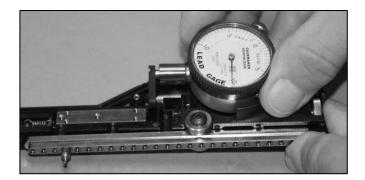
6. Replace the contact point in the new indicator with the contact point from the old indicator.
