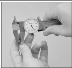
4. Install a contact point into the moveable holder at the front of the gage.
