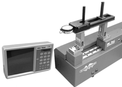
Zeroing the MRP-5000 with the MIC TRAC Setting Master (Diagram 9)
