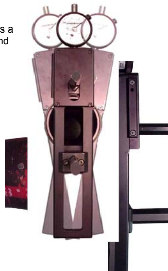
The gage contacts the face of the connector as the rolls seat into
