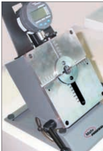
Measuring thin-sheet-formed components such as aluminum cans can be a self-defeating process since they may distort while being measured. In these cases special tooling will help to round-up the part to enable accurate measurement.
