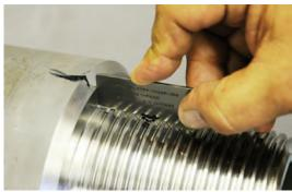
7. The connection is now properly marked and ready to measure the pitch diameter using the PD-8000-RSC gage.
