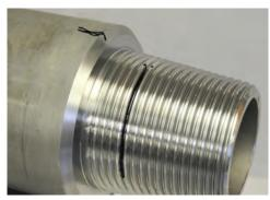
Measuring the Pitch Diameter of the Pin Connector
