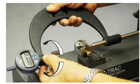
5. With the indicator on the bottom side of the connector, place the fixed contact ball at the point where the LPP was located and marked.
