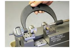
2. To preset the gage, loosen the lower arm lock screw and slide it to the approximate location where the standard will fit between the contact points.
