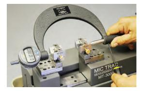
4. Place the standard between the contact points, sweep the standard in a small circular motion to locate the smallest reading and zero the indicator.
