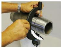
The reading on the indicator is the amount of deviation from the nominal pitch diameter.
