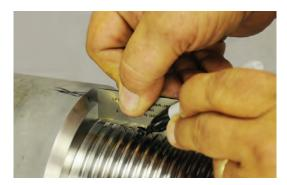
6. Repeat steps 4 and 5 to verify proper template location. Holding the template **firmly** into the threads will ensure the left edge is parallel and square against the pin shoulder.
