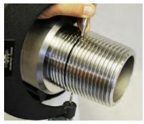
7. While holding the fixed contact ball at the marked location, sweep the gage to locate the largest indicator reading.
