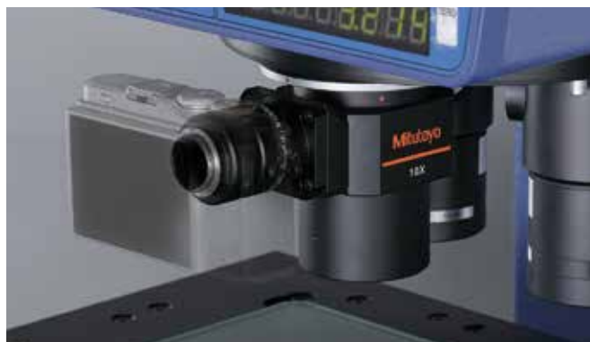
Example of attaching the Projection Lens 10X with C mount on PJ-H30
