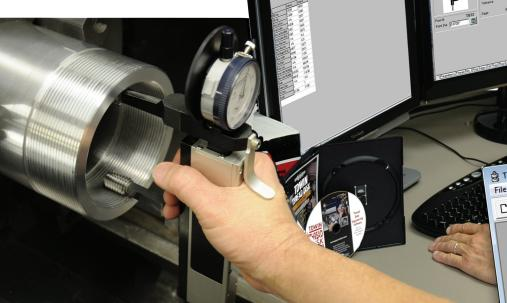
The Thread Data software calculates critical dimensions for threads based on ANSI tables and formulas.
