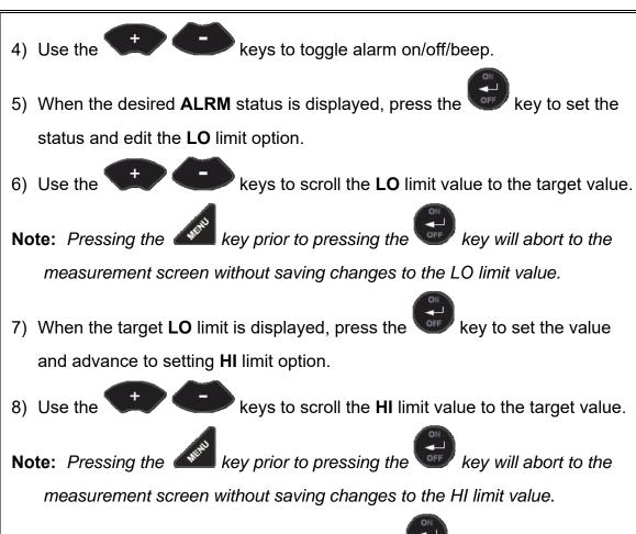
9) When the target **HI** limit is displayed, press the and return to the measurement screen.
