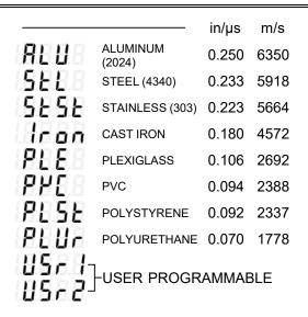
3) When the desired **MATL** setting is displayed, press the wey to set the material velocity and return to the measurement screen.
