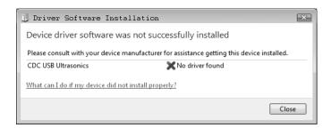
The driver file that needs to be installed can be downloaded directly from our website at <a href="www.dakotaultrasonics.comDUsoftware/CDC/CDC\_Ultrasonics.inf">www.dakotaultrasonics.comDUsoftware/CDC/CDC\_Ultrasonics.inf</a>, or can be found in the examples folder created on your PC by installing our DakView PC software, and located in the USB directory. The file name is CDC\_Ultrasonics.inf, and can be downloaded and saved anywhere on your local PC.
