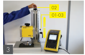
3 Adjust height of the marking head (tighten the locking handle (1), adjust height with the upper wheel (2), release the locking handle (3) then lock it
