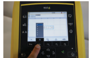
9 Press "force" key and select 1 to 6 (intermediate setting is 2)
