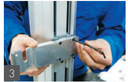
3 Fix the fixing plate on the column (see assembly plan ASC10 included in the packing box).
