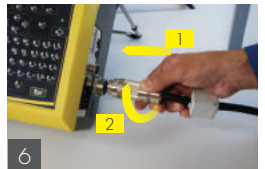
6 Connect the marking-head cable to the controller (1), and lock it (2).
