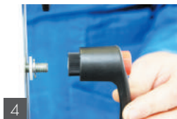
4 Tighten the locking handle on the column (see assembly plan ASC10 included in the packing box).
