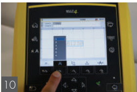
10 Select key: "character dimension" and adjust height/width with arrows
