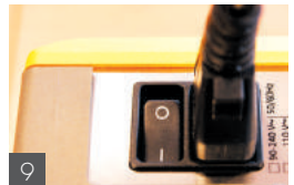
9 Power up the machine by switching the main switch to (I).
