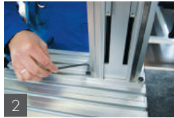
2 Assemble the base and the column (see assembly plan ASC10 included in the packing box).
