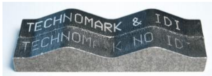
Marking with IDI curved mode and without IDI
