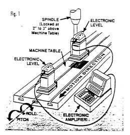
For final qualification, B5.54 calls for a high degree of repetition. Tests are run with the table traversed in both directions, after which the levels are turned 180\_ and the table is again traversed in both directions. Because of the ease of using electronic levels, this redundant testing can be accomplished quite quickly.
