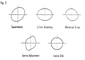
Note that the ball bar is primarily a test of contouring performance. Other tests can be run to check repeatability and Hysteresis. However, because of its short measurement range (about .080"), it is not an effective tool to check linear or volumetric accuracy over the machine's range of
