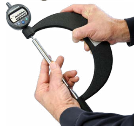
Setting PD-8001-RSC with Rod Standard
