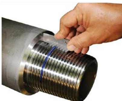
LPP on a Pin with blue line marking proper thread
