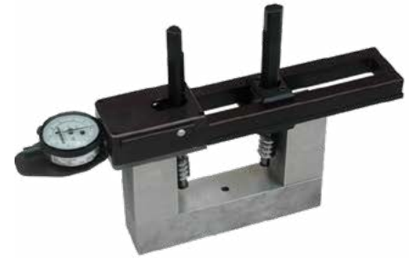
Setting an MRP-5001 with Frame Style Standards
