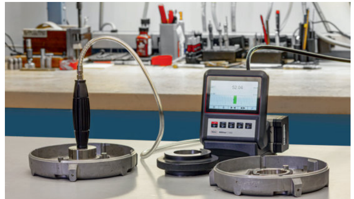
Stand alone air gaging for bore diameter
