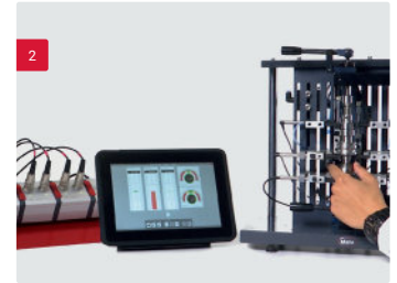
Shaft measurement with inductive modules
