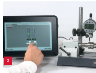
Radial run out measurement with dial indicator
